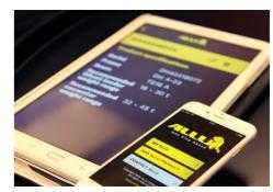
the right angle of inclination used by the ALLU Transformer. In order to maintain maximum productivity on the site and to minimise equipment downtime, the ALLU App provides information about the ideal maintenance frequency and the changing of wear parts, based on the number of working hours. Furthermore, The ALLU App provides instructions to guide the operator through safe working methods when using the ALLU attachment throughout the whole operating and ownership process.
