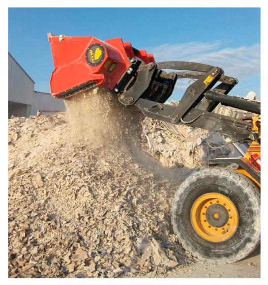
Blade thicknesses determine the fragment size of the end-product and ALLU has a range of blades than can easily be changed onsite to produce required fragment sizes.
