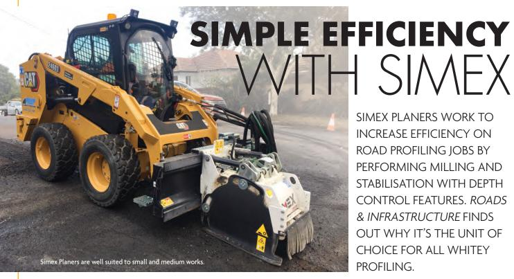
SIMEX PLANERS WORK TO **INCREASE EFFICIENCY ON** ROAD PROFILING JOBS BY PERFORMING MILLING AND STABILISATION WITH DEPTH CONTROL FEATURES. ROADS & INFRASTRUCTURE FINDS OUT WHY IT'S THE UNIT OF CHOICE FOR ALL WHITEY PROFILING.
